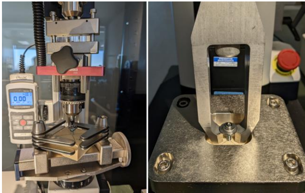
Figure 3: Screw insertion with Mark-10 TSTM-DC-1 (left) and screw pullout with Mark-10 ESM303 (right).
